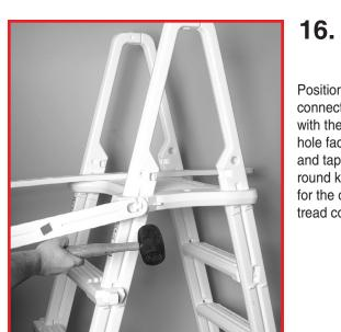
Position the tread connector as shown, with the padlock hole facing upward, and tap it over the round knob. Repeat for the opposite tread connector.
