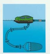
The pressure of clean water returning to your pool powers the Turbo Turtle, leaving both the filter and skimmer free to eliminate contaminants.
